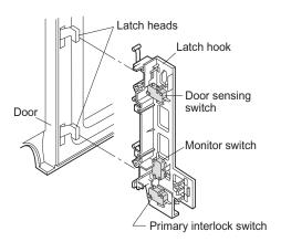
Figure D-1. Door Open Mechanism
